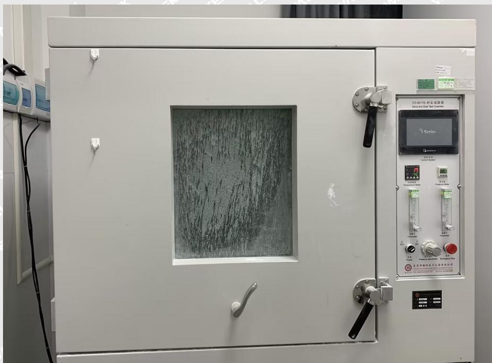
During the IP 6X test
