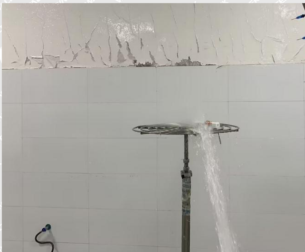
During the IP X6 test
